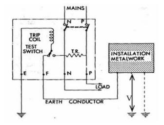
Short for Earth Leakage Current Breaker. Detects if electricity is leaking to earth from an appliance. Protects from shocks. Has a trip coil. Trips when voltage difference between the frame earth and the reference earth exceeds the rated voltage (usually 40 V). The trip coil is energized by the voltage difference, and the spring-loaded contact is released which breaks the circuit and cuts off power. Up to about 50 V has been traditionally considered as a safe voltage.
