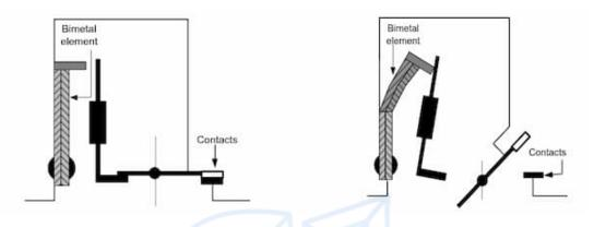
Consists of a bi-metal strip. When overheated from overload current, the bi-metal strip is deflected. The deflection depends on the heat which depends on:
