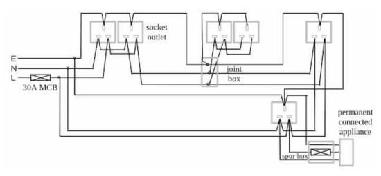
Each circuit commences from consumer unit through an MCB (or fuse), loops into each socket outlet and returns to the same MCB (or fuse) in the consumer unit.
