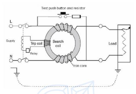
Short for Residual Current Device. Protects against electric shock and fire risks.
