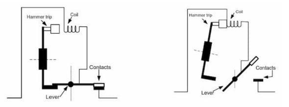
Consists of a solenoid coil. Load current is set to flow through the coil.
