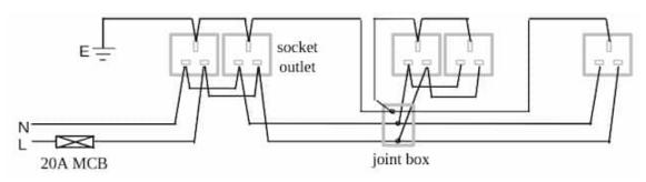
Each circuit commences from consumer unit through an MCB (or fuse), loops into each socket outlet and terminates at the last socket outlet.
