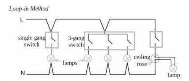
Enables all joints and terminations in a single final circuit to be made at ceiling roses, switches or other accessories. This makes all joints accessible for testing and alterations. Each final circuit has both its live and neutral conductors terminating at the consumer unit. Wires are usually laid in PVC conduits.
