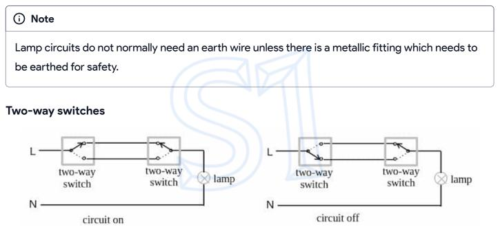
Used when it's necessary to operate an equipment from 2 positions.
