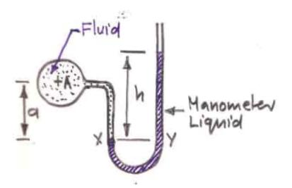
Hydrostatic principle is used here. Measures absolute pressue. Manometer liquid should not mix with the liquid in which the pressure is to be measured.
