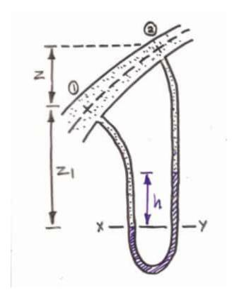
Used to measure pressure difference between two points. Can be used for both liquids and gases. Difficult to measure small pressure differences (because small displacement of manometer liquid).
