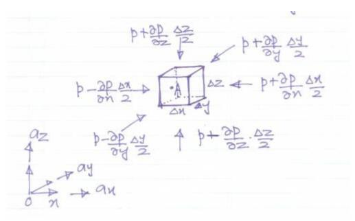
By applying Newton's second law of motion in all 3 directions:
