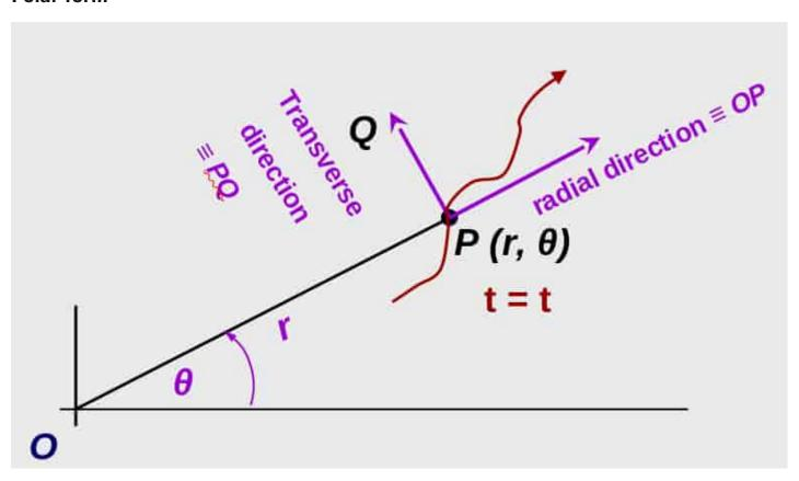
Velocity have a transverse and radial components.
