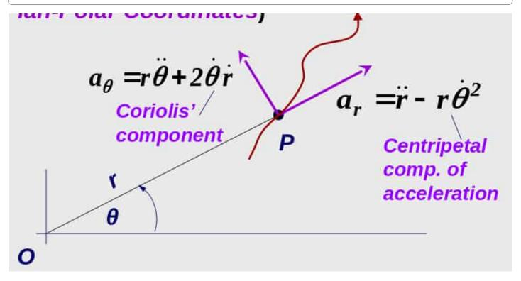
Acceleration also have a transverse and radial components.
