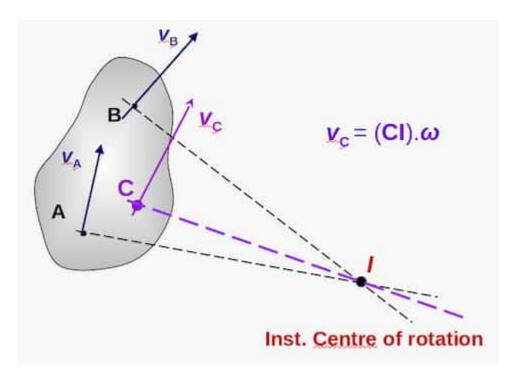
${\it I}$  can be found by drawing a line perpendicular at the velocity vectors at 2 different points and finding their intersection point.
