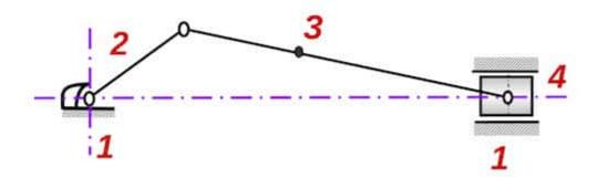
For example, in slider crank mechanism:
