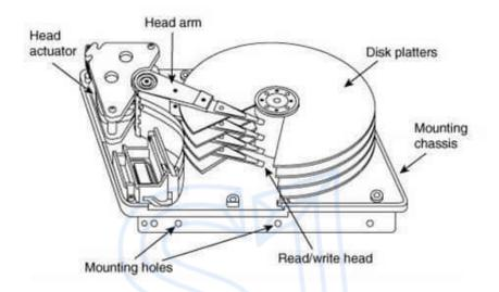
Capacity can be improved by adding more platters. Platters are kept in dust free environment to avoid damages because of high speed. Each side of the platter require a read/write head.
