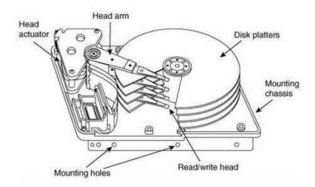
Capacity can be improved by adding more platters. Platters are kept in dust free environment to avoid damages because of high speed. Each side of the platter require a read/write head.
