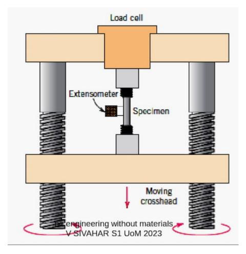
Test will be done until the specimen fractures. Results are converted to engineering stress and strain, and plotted.
