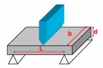
Support the material at 2 ends. Apply pressure perpendicular to the material until the material fractures.
